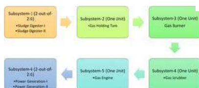
Fig 1. Configuration diagram of power generating unit. https://doi.org/10.1371/journal.pone.0284848.g001
